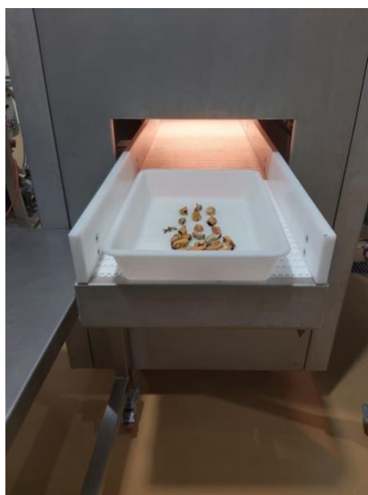
Figure 4. Mussel test in Hypespectral system
